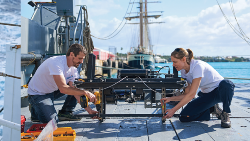
Above: Leo Blanco-Bercial and Amy Maas, assistant professors, assemble the Multiple Opening and Closing Net and Environmental Sensing System to collect zooplankton at various ocean depths.
